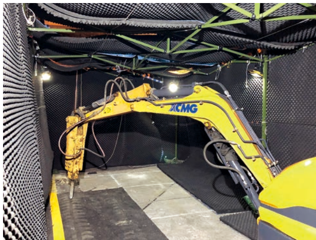
The remote-controlled Little Swan excavator, which is equipped with a mobile muffler box, minimises noise at sites and makes night-time roadworks more efficient.
